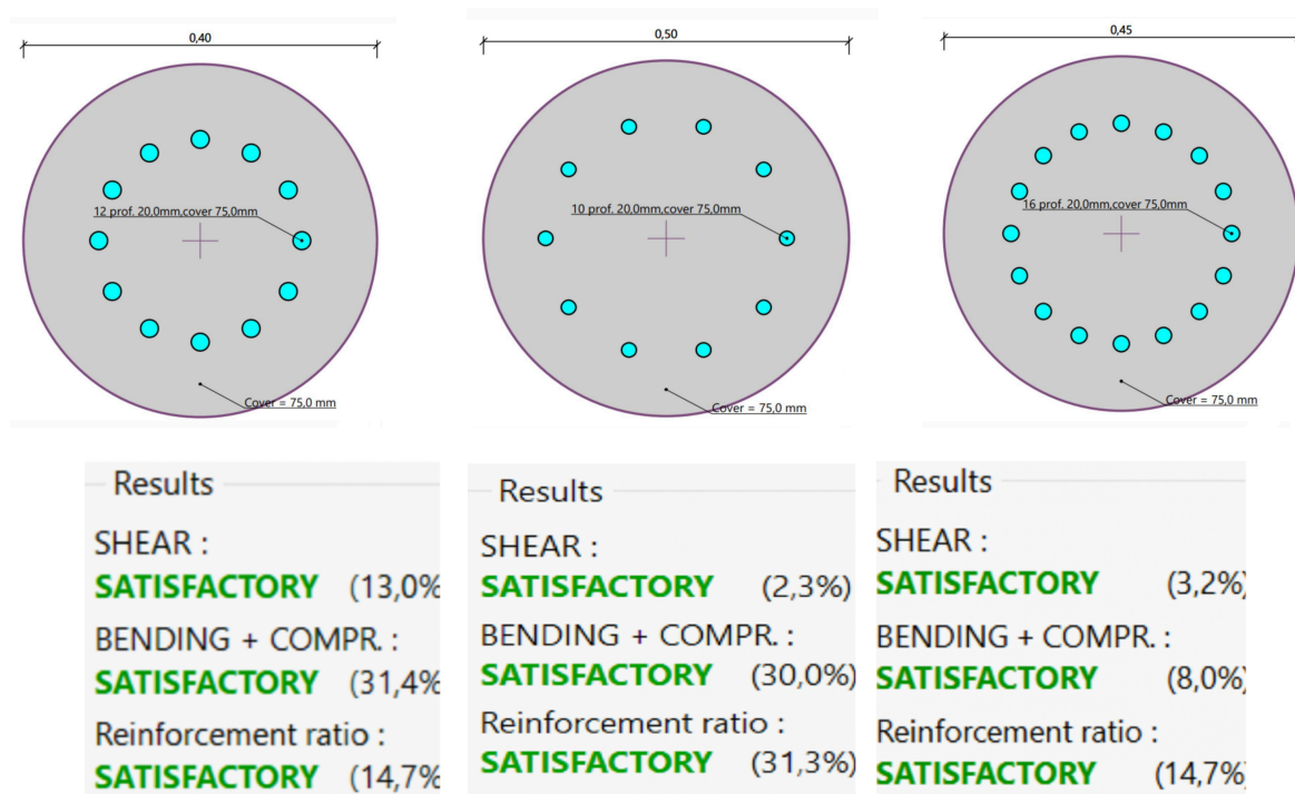
Figure 4.3.4.2.1 The reinforcement patterns for single piles depend on their group location (exterior, interior, or corner).
