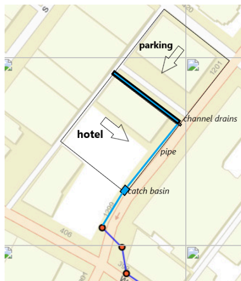
Figure 5.3.1 Preliminary layout of the storm sewer system
