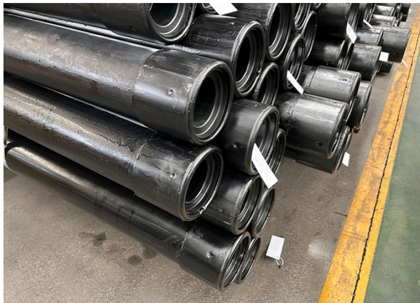
Figure 5.1.12. Tubing with corrosion resistant alloys
