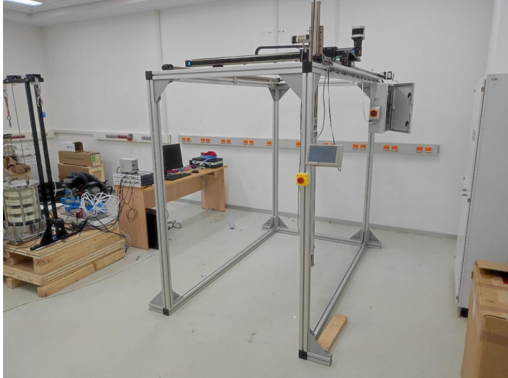
Figure 13: 3D Construction Printer
