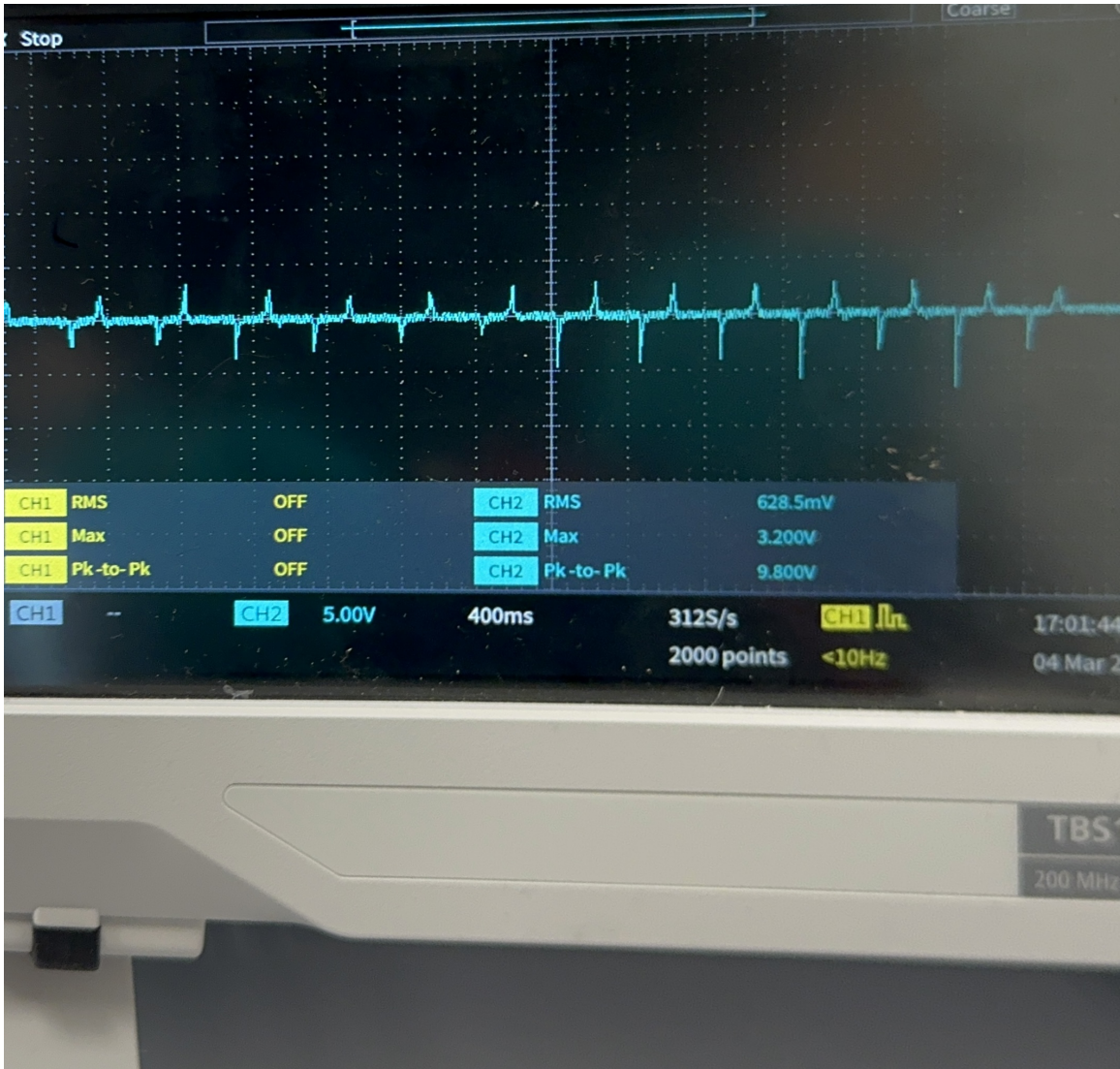
Figure 3-2: Generated signal values on TENG sensor during continuous impacts.
