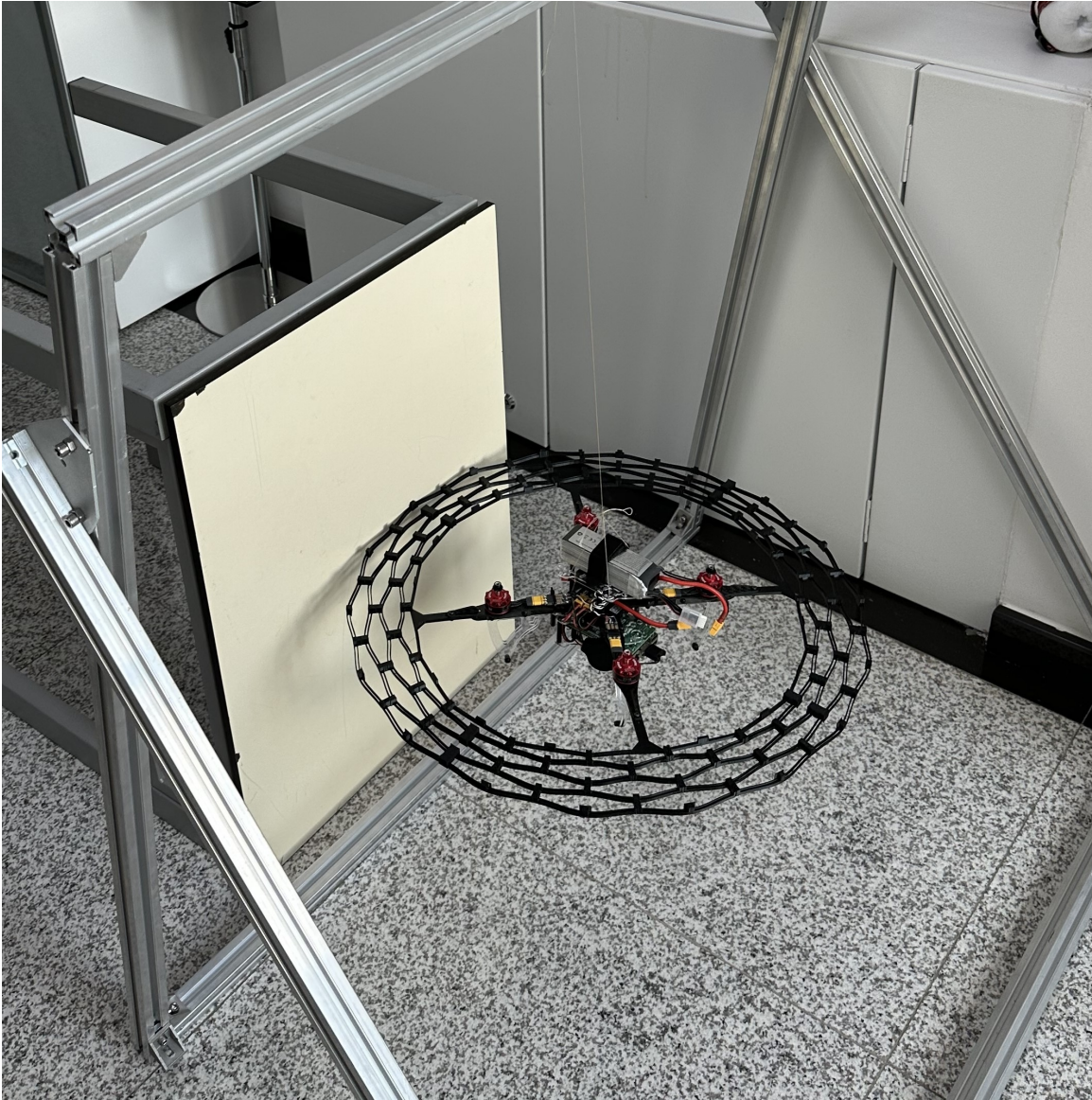
Figure 4-2: Pendulum test setup and an implemented OrbiComb structure around the Coex Clover 4.2 drone.
