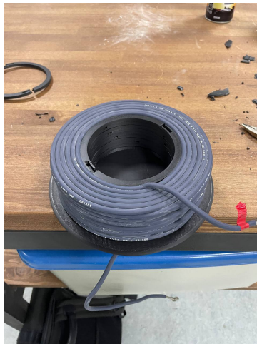
Figure 3.8: Assembled modular air-core transformer.
