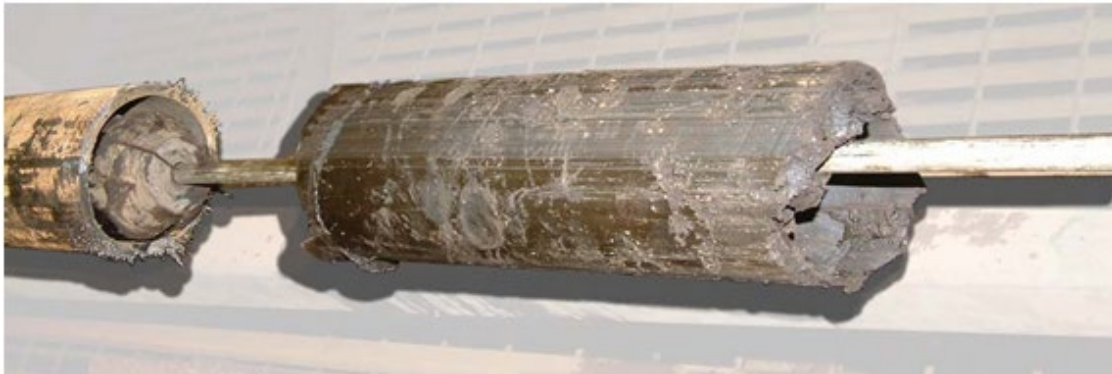
Figure 1.1. Wax sample recovered with sucker rod during tubing replacement (Bellarby, 2009)
