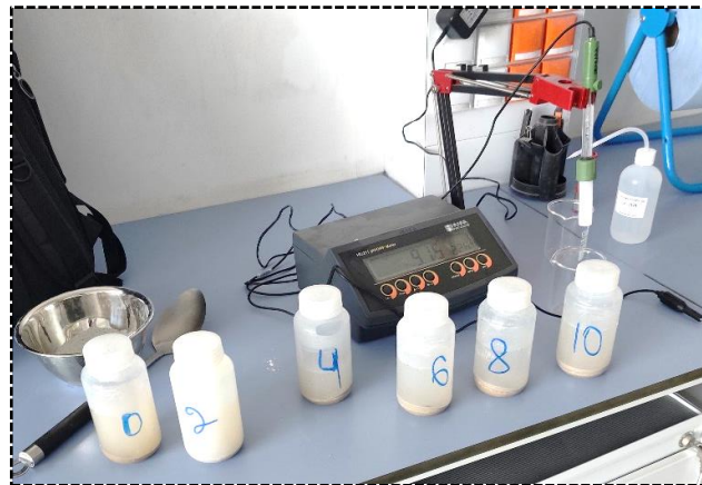
Figure 3.6 Setup of Eades-Grim Test for determining the standard lime content.
