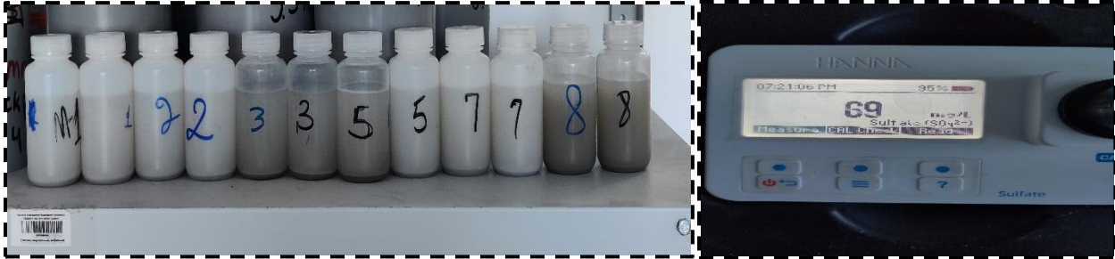
Figure 3.8 Set up of Colorimetric test for determination of soluble sulfate concentration.
