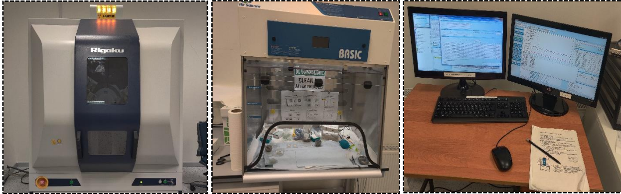
Figure 3.15 Setup for X-Ray Diffraction Test
