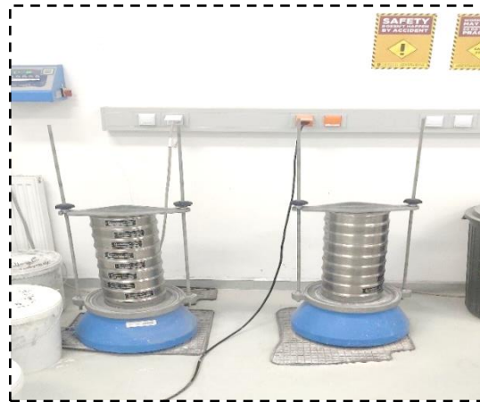
Figure 3.4 Setup of Soil Gradation (Particle Size Distribution)
