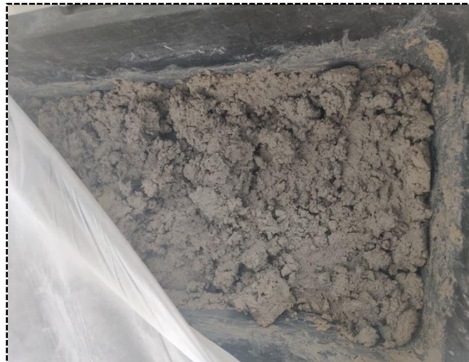
Figure 3.10 Soil Mellowing Process.
