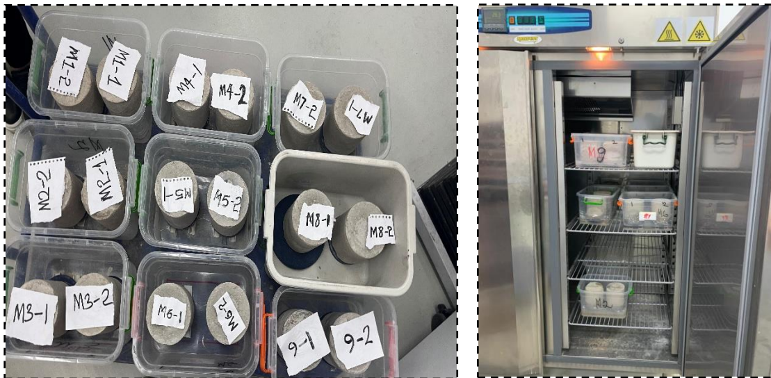
Figure 3.13 Setup of Freezing-Thawing Test for 60 cycles action.
