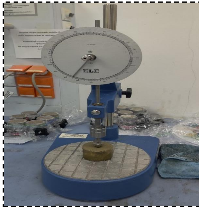
Figure 3.3 Setup of cone penetrometer for liquid limit determination
