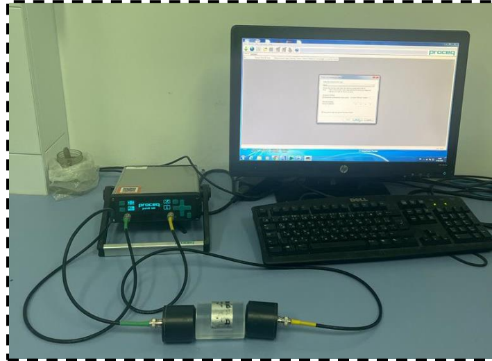
Figure 3.14 Setup for Ultrasonic Pulse Velocity (UPV) Test.
