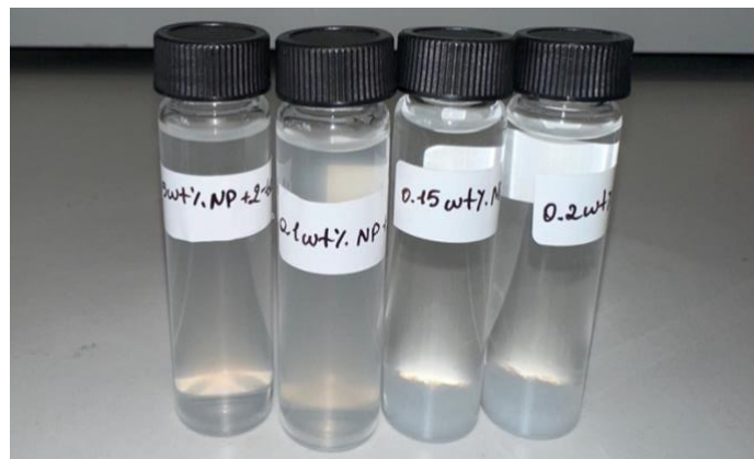
Figure 16. Aqueous stability test for NPs in LSW
