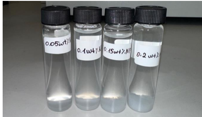
Figure 15. Aqueous stability test for NPs in SW
