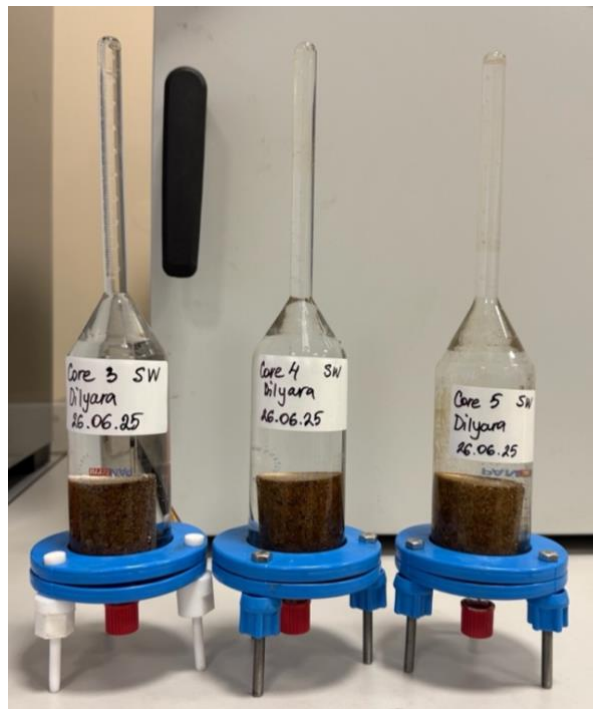
Figure 13. Representative SI experiments conducted in Amott cells
