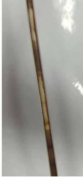
Figure 27. Observed process, of foam pushing out the out, in transparent tube installed on outlet line
