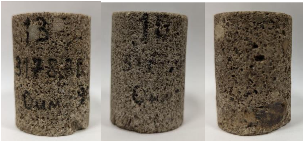
Figure 21. Oilfield “X” reservoir core plugs used in coreflood experiments.
