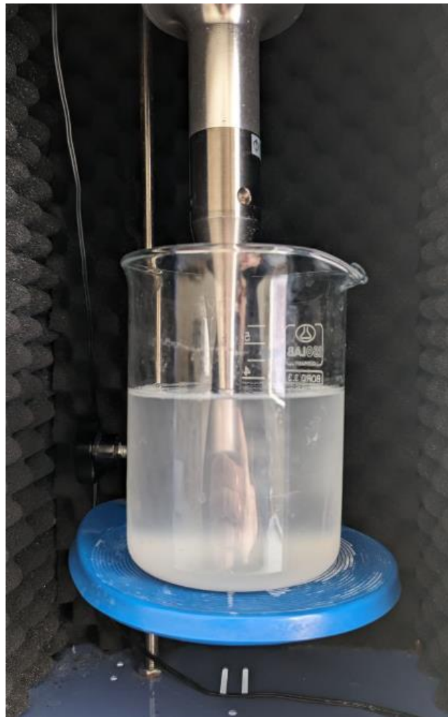
Figure 17. Photo of homogenizer application to prepare nanoparticle (np) solutions
