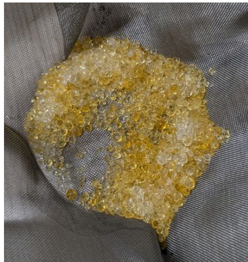
Figure 25. Silica gel sample after 5 hours in the dryer
