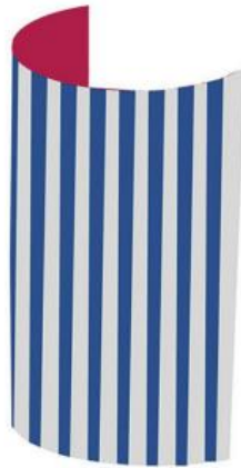
Figure 4. The flexible MTM absorber for X-band application [23].
