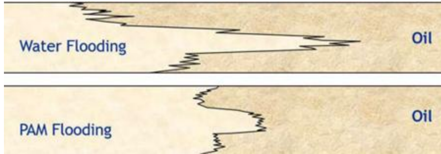
Figure 4. Water fingering illustration (Jones et al., 1984)
