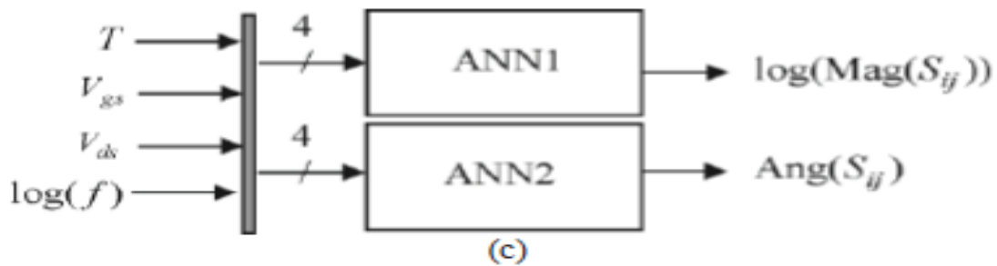
Fig. B1. Model studied for GaN HEMT (a) Equivalent circuit model (b) neural model for S_{11} , S_{12} and S_{22} (c) neural model for S_{21}
