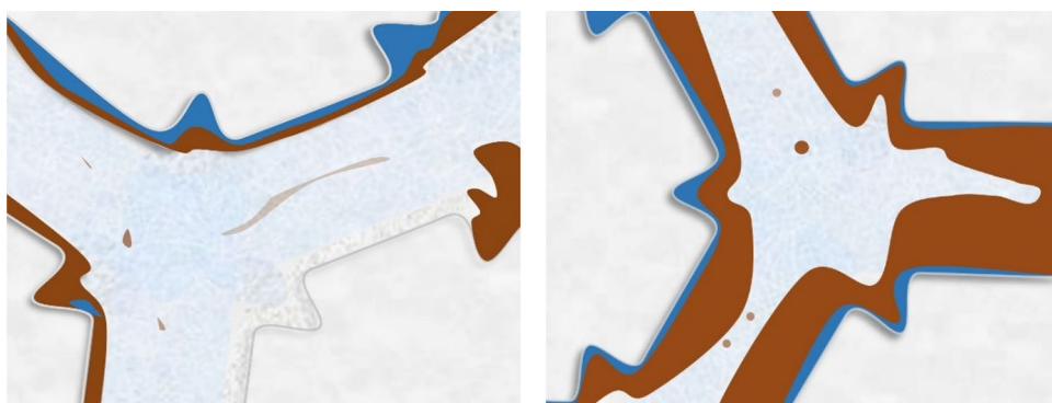
Fig. 6 Microscopic analysis of surfactant flooding in left water-wet medium and right oil-wet medium. The deep blue is representative of the formation brine, the brown represents the oil, and the white represents the surfactant solution (Yadali Jamaloei and Kharrat 2009 adapted from Yadali Jamaloei and Kharrat (2009))
