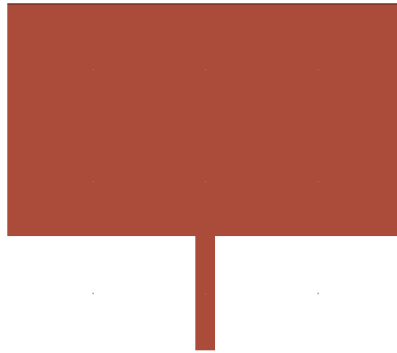
Figure 3.1: Rectangular patch antenna structure.
