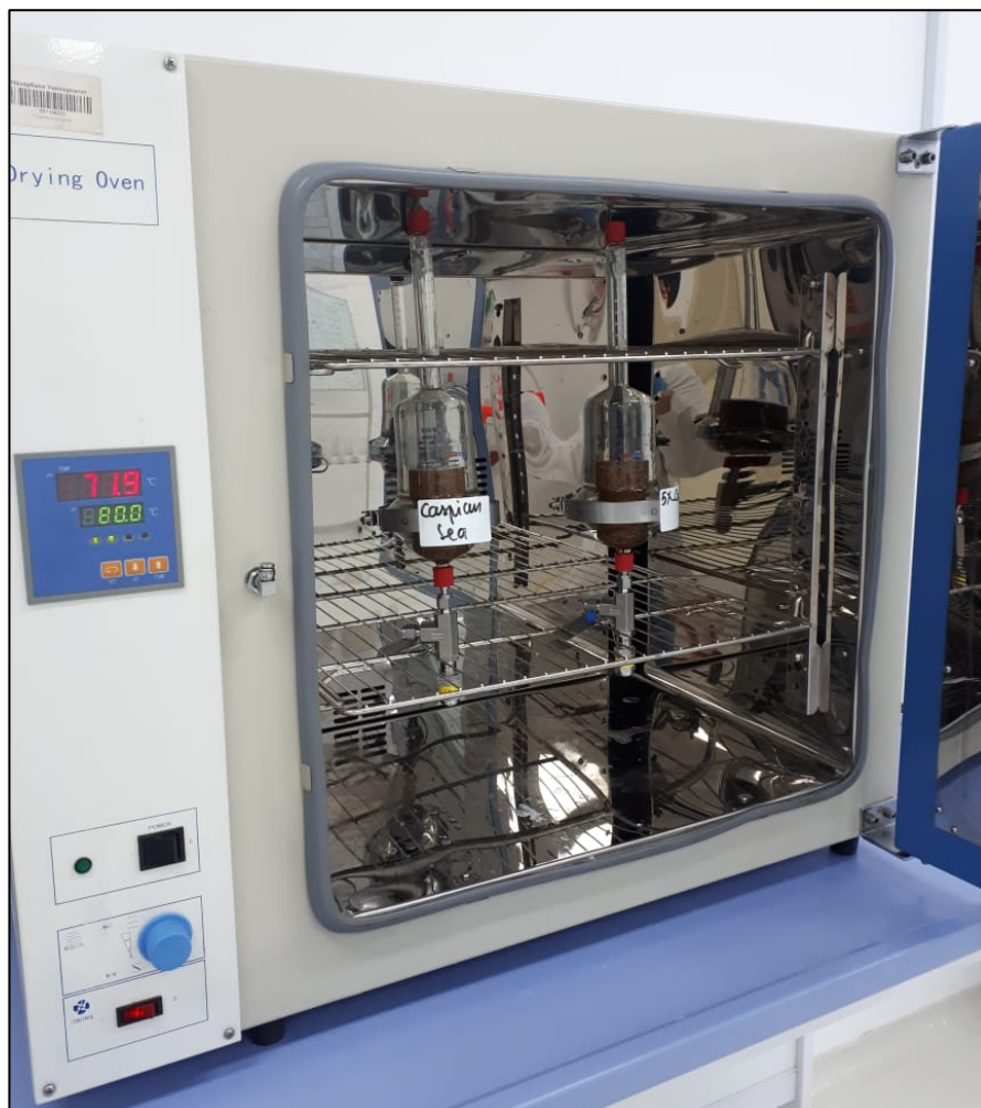
Figure 24. Spontaneous imbibition test in the lab
