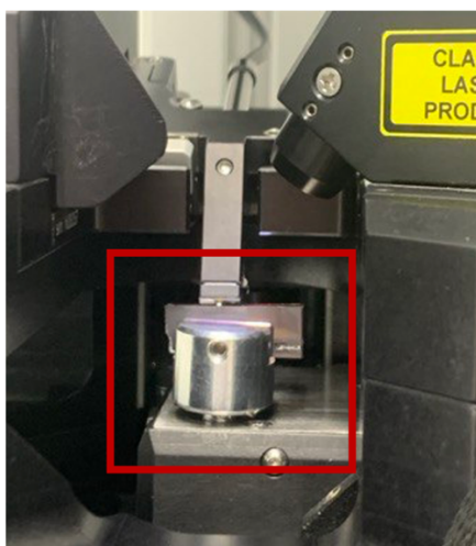
Figure 3.17 Adapted cross-section sample holder for the AFM instrument
