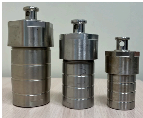
Figure 4.1 Teflon-lined autoclaves of 100, 50, and 25 mL capacity employed for solvothermal synthesis
