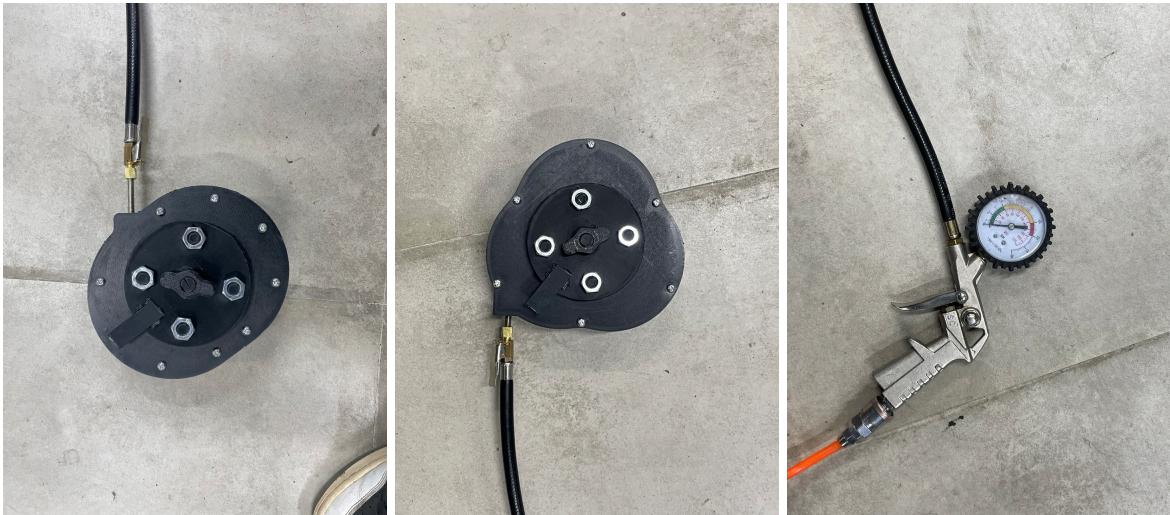
Figure 22. 3D printed Wankel and LiquidPiston engines connected to compressor
