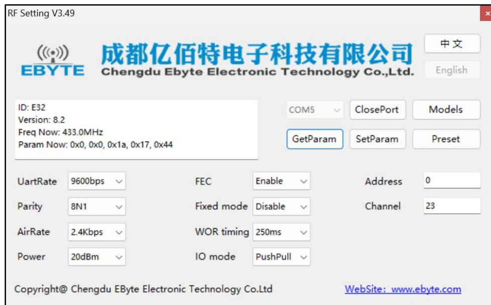
VEV-4. Configuring the LoRa module. Transmit power and air data rate can be changed.
