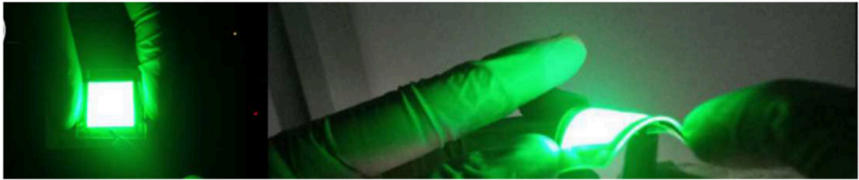
Figure 2.3. Photos of flexible LED based on SCQDs [22]
