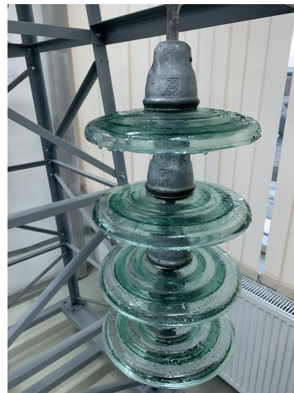
(b) Glass insulator
