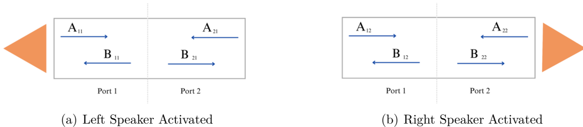
Figure 1: 1D Acoustic Waveguide Working Principle
