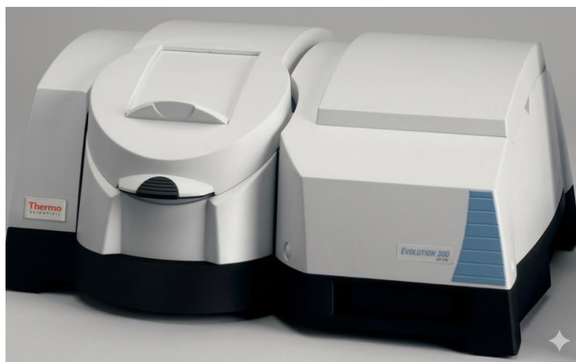
Figure 8. Thermo Scientific Evolution 300 UV-Vis spectrophotometer used for effluent sample analysis
