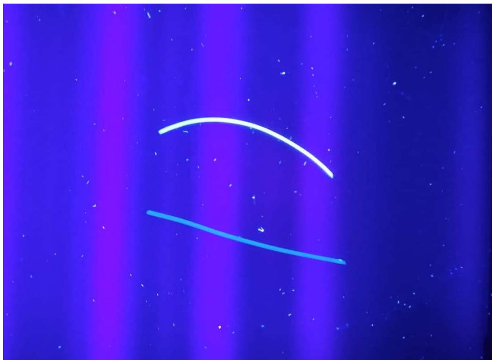
Figure 3.2 Polymer rods examined with UV lamp: drug-loaded (top) and drug-free samples (below)
