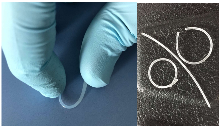
Figure 3.1 Bended wet and circled dry polymer rods performing excellent mechanical properties
