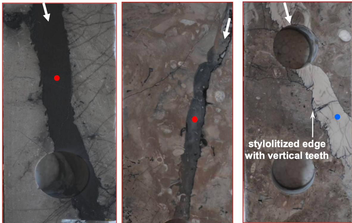
Figure 4. Photo of a Type A fracture observed in core sheds at Tengiz. Adapted from Cook et al. (2002).
