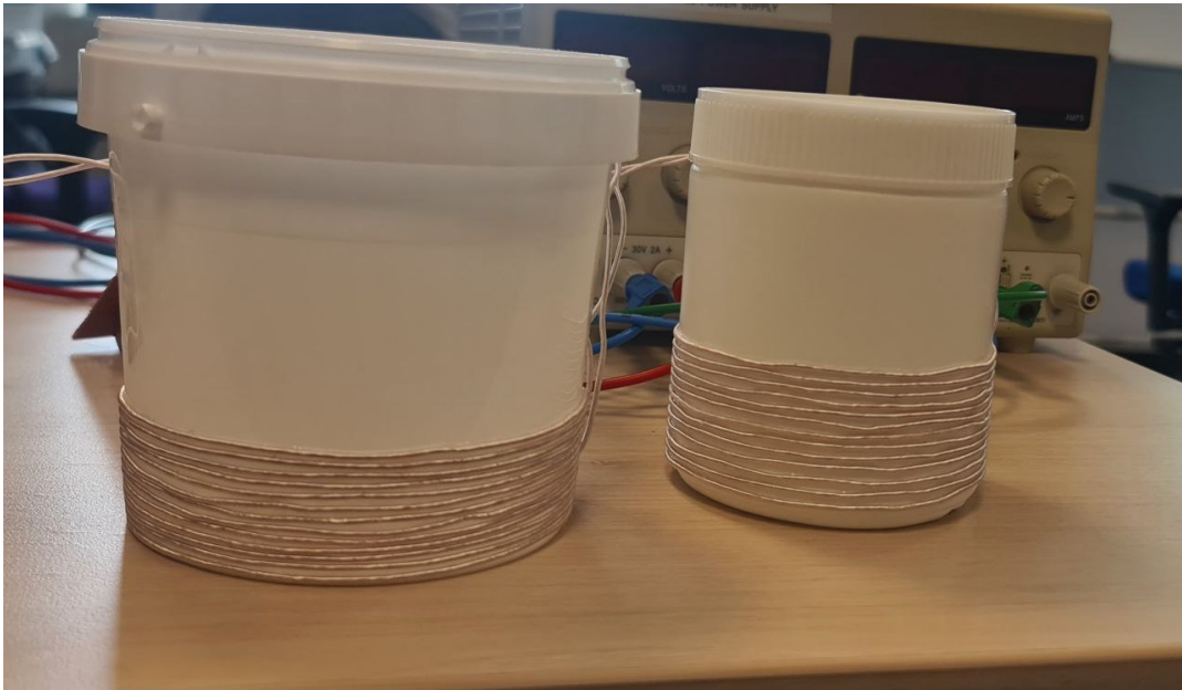
Figure 5.2: Designed Concentric Coils
