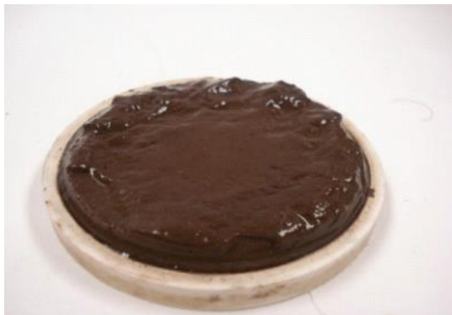
Fig. 7. Ceramic disc with formulated filter cake (Rostami & Nasr-El-Din, 2010)
