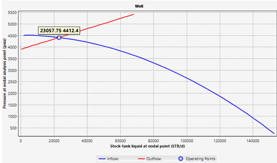
Figure 99. Operating point for water injection well.
