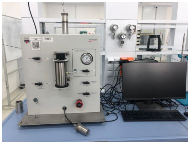
Figure 22. Vinci HEP-P Helium Porosimeter
