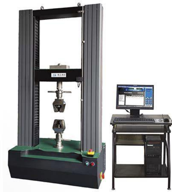
Figure 17. Model CMT5105 microcomputer-controlled Electronic Universal Testing Machine.
