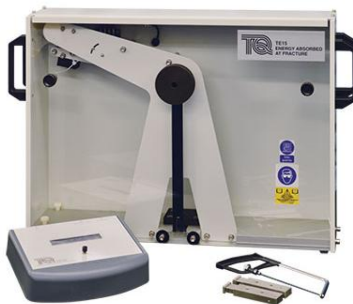
Figure 20. TecQuipment TE15 Energy Absorbed at Fracture machine [47].
