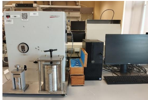
Figure 10. Helium Porosimeter to measure the core porosity
