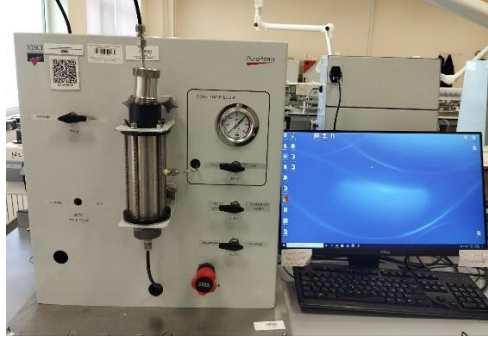
Figure 11. PoroPerm apparatus to measure the core permeability
