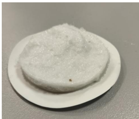
Figure 9. Salt precipitated from the HSW after filtration
