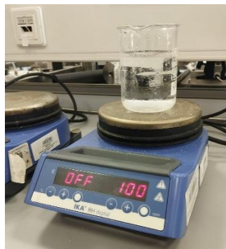
Figure 12. Magnetic stirrer used to mix solutions
