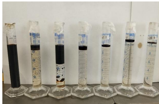
Figure 40. Surfactant flooding profile (a) pressure drops, (b) fluid production, (c) inlet and outlet differences, and (d) effluent samples collected during the flooding
