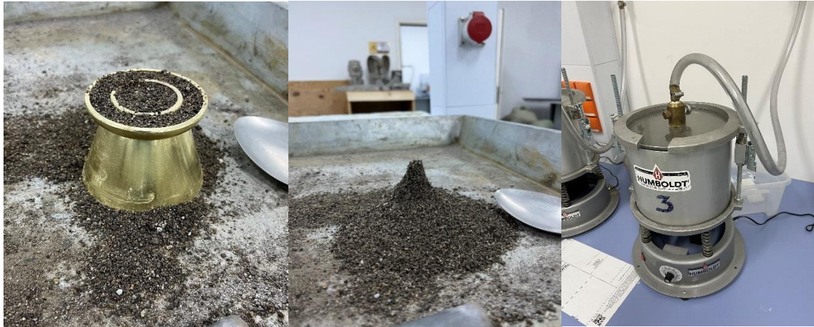
Figure 3.7: Procedure of determining SG and AC of aggregate materials
