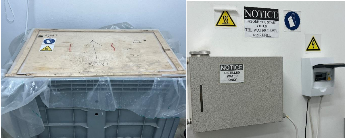
Figure 3.11: Steam curing chamber and steam generator
