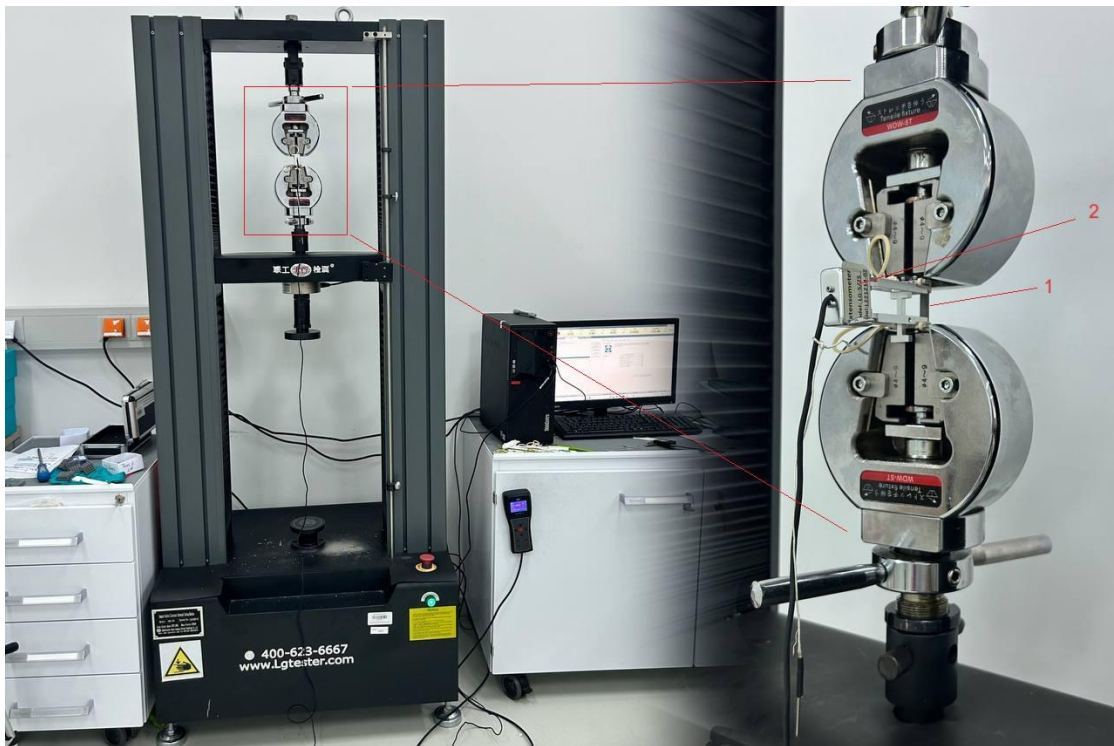
Figure 3.2: Tensile test setup: 1 - sample, 2 - extensometer
