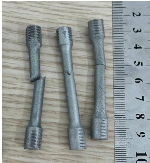
Figure 4.5: Tensile results of the Ti-6Al-4V samples
