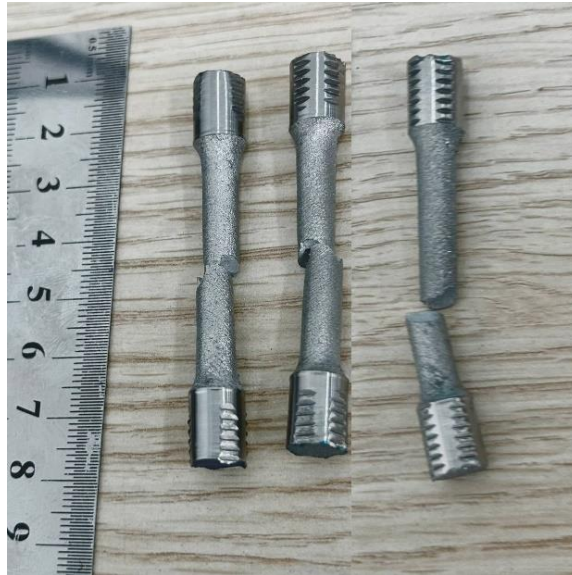
Figure 4.8: Tensile results of the Ti-6Al-4V-Ta samples
