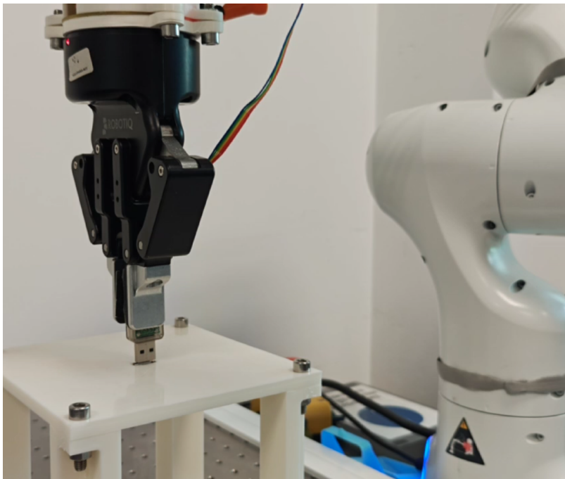
Figure 5-1: The setup with 15x15cm platform to hold USB hole
