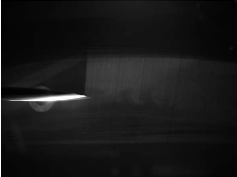
Figure A.8: Non-inverted PIV image of the particle flow around the serrated wing at 3 m/s
