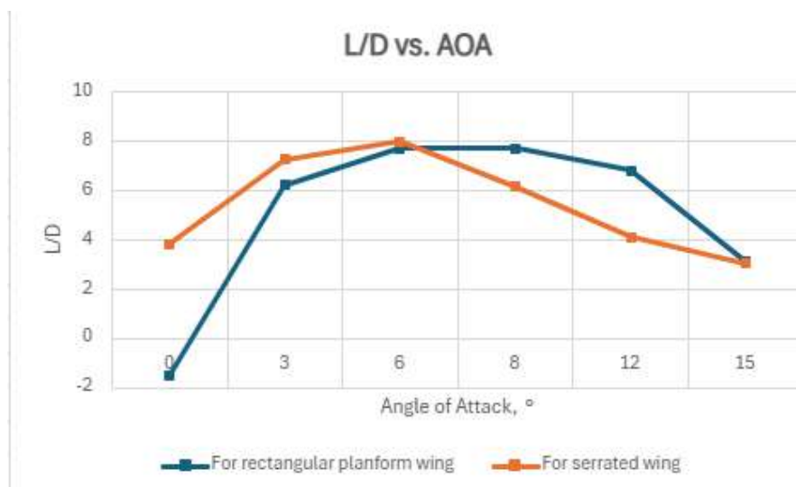
Figure 4.9: Ratio of lift to drag vs Angle of Attack for both wings
