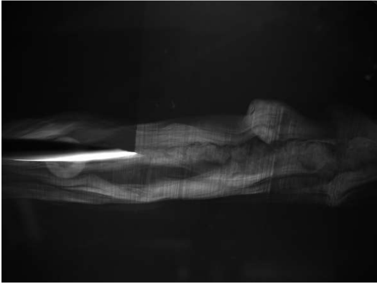
Figure A.11: Non-inverted PIV image of the particle flow around the serrated wing at 6 m/s
