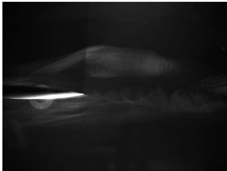
Figure A.10: Non-inverted PIV image of the particle flow around the serrated wing at 5 m/s
