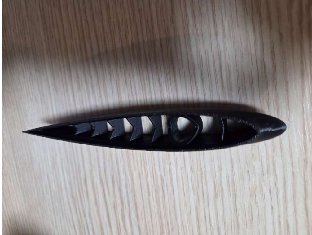
Figure 3.15: Bridge like Structure for 3D Printing
