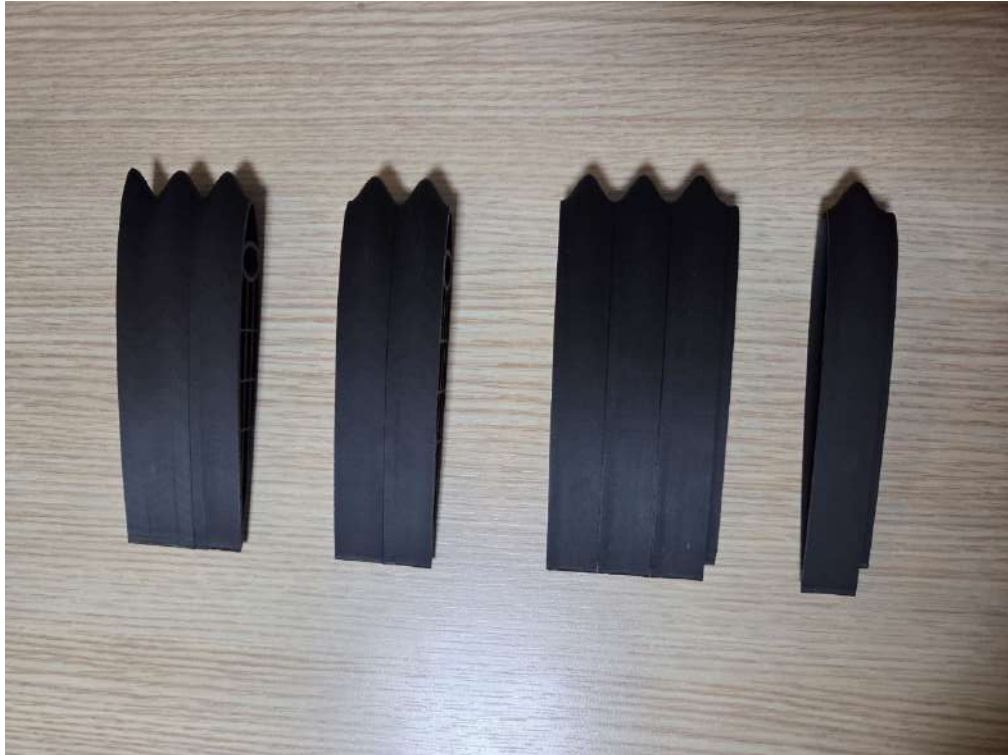
Figure 3.14: Attempts at Printing Serrated Wing
