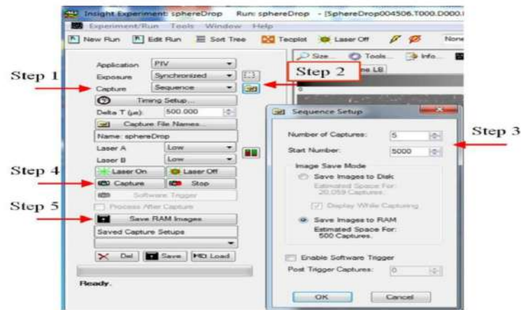
Figure 3.8: Image Capturing Setup
