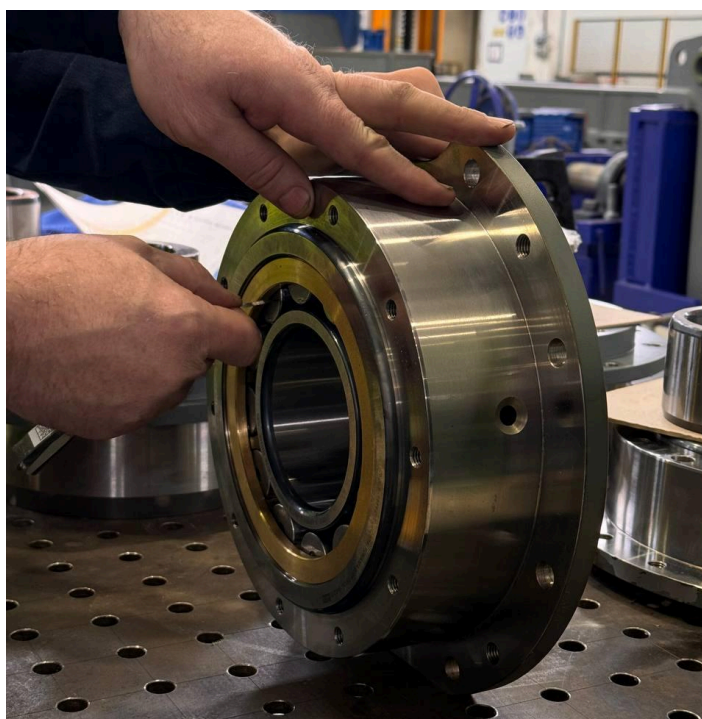
Figure 16. The Process of Measuring the Bearing Clearance
