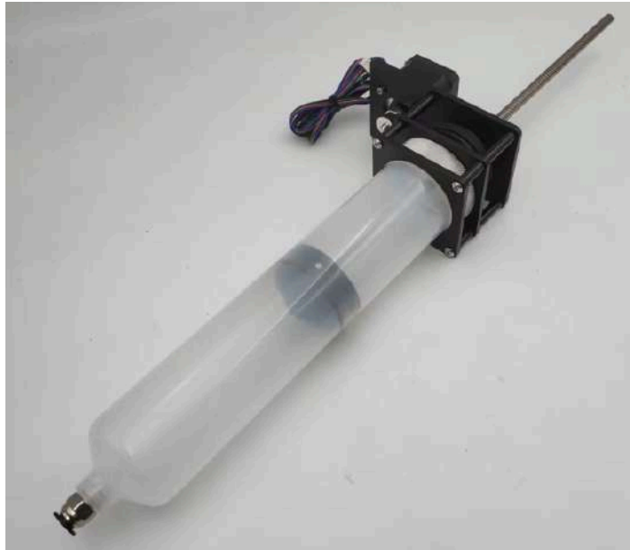
Figure 9. Example of screw-driven pumping system [8].
