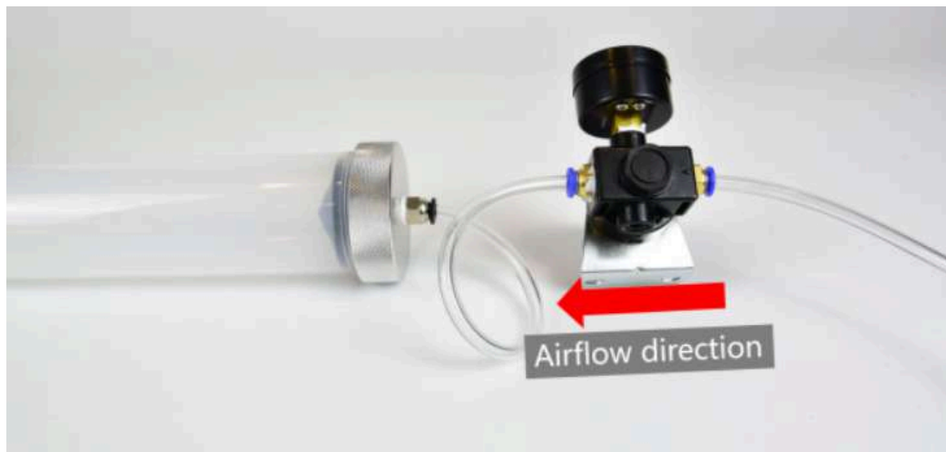
Figure 8. Pneumatic Pumping system example [8].
