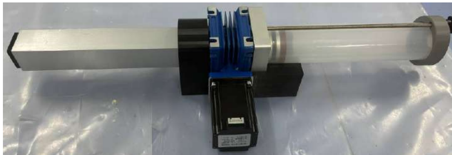
Figure 17. Assembly result of pumping system
