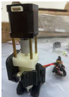
Figure 18. Extruder with a holder
