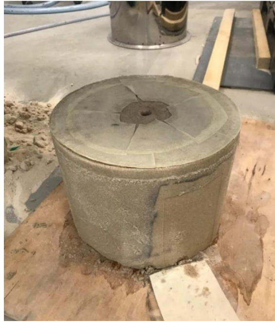
Figure 5.9. Experimental sample after sand production (Kozhagulova et al., 2021)
