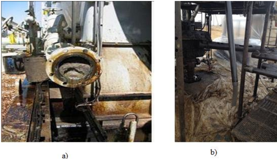
Figure 2.1. Sand production problems in the oil field. a) Surface pipeline clogging; b) Clogging of tubing
