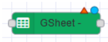
Figure 3-9: GSheet node integrates Node-RED with Google Sheets via the Google Sheets API, allowing flows to programmatically read from and write to cloud-based spreadsheets.
