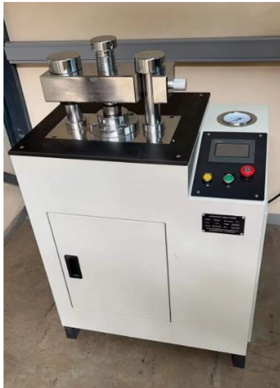
Figure 3-11. Auto Pallet Press Machine
