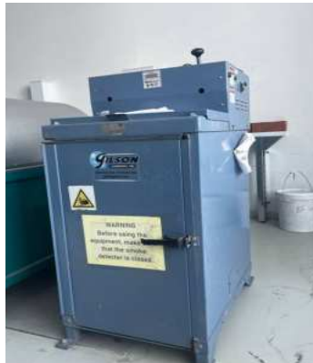
Figure 3.2. High-Capacity Sieve Shaker used for BOFS Sieving.
