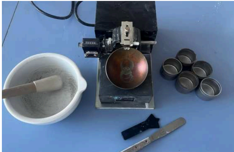
Figure 3.8. Atterberg limits apparatus.
