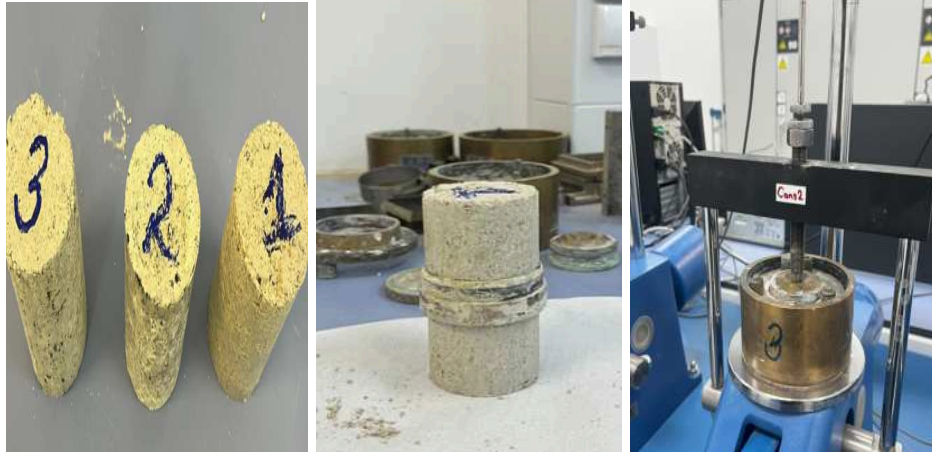
3.13. Sample preparation for consolidation test.
