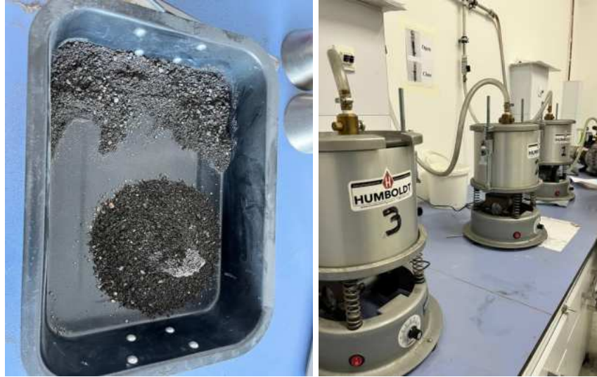
Figure 3.4. Specific gravity test of BOFS materials.
