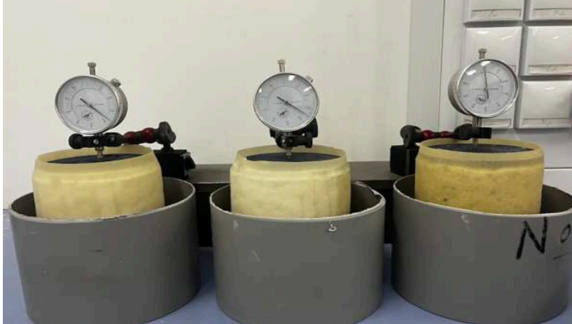
Figure 3.17. Dial gauge setup for vertical expansion measurement.
