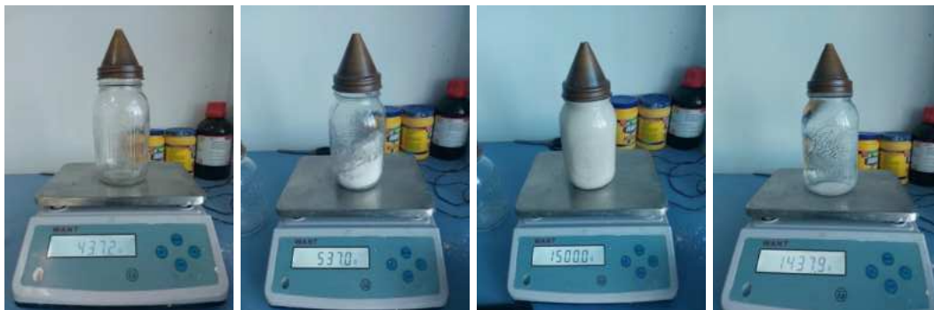
Figure 3.10. Specific gravity test procedure of kaolin clay.
