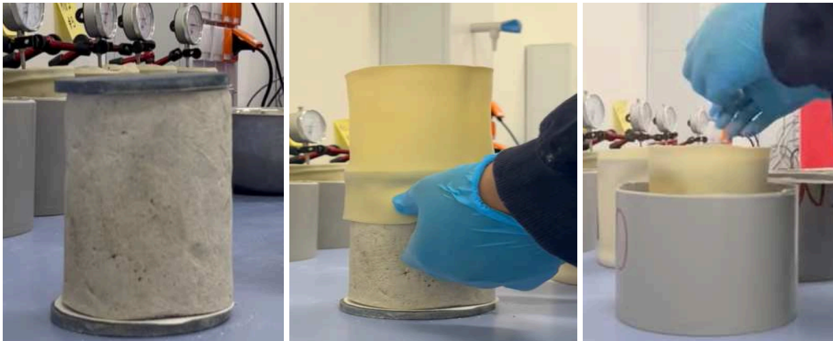
Figure 3.16. Sample installation procedure for the swelling test.
