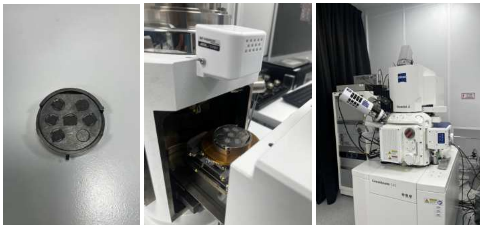
Figure 3.19. SEM analysis equipment.
