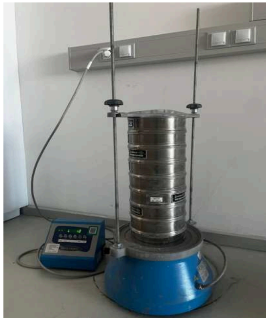
Figure 3.6. Mechanical sieve shaker used for soil sieving.
