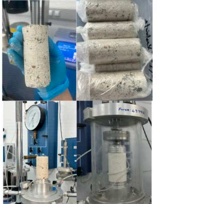
Figure 3.14. Unconfined compressive strength test process.
