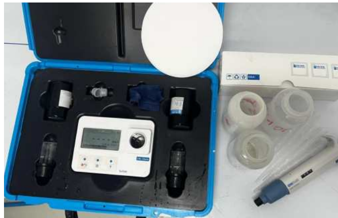
Figure 3.9. Sulfate content measurement test kit.
