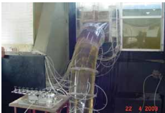
Fig. 3 Lines of pressure (experimental/numerical) gauge stations
