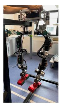
As we mentioned, we had two ways of dataset collection and testing of NN. These are the CoppeliaSim model and physical prototype. We decided to focus on the left leg of bipedal robots. Thus, we will be able to do the research faster as if we did for both legs we would have to always change the code second leg and consider one leg hitting another. The left leg has 6 joints. Therefore, we will gather data and train NN for the supply of torque for these 6 joints
