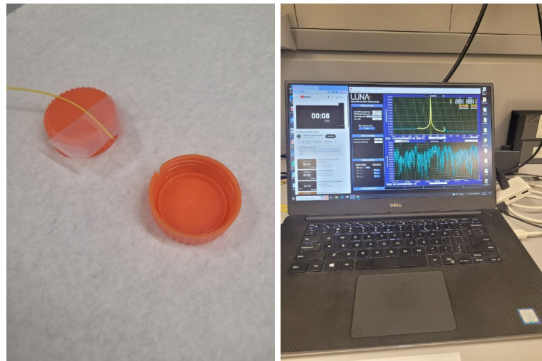
(a) Immersing of SDI into sucrose solution (b) LUNA 4600 OBR measurements
