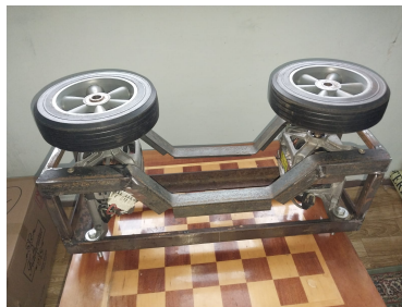
Figure 4.4: Main body with wheels and motors
