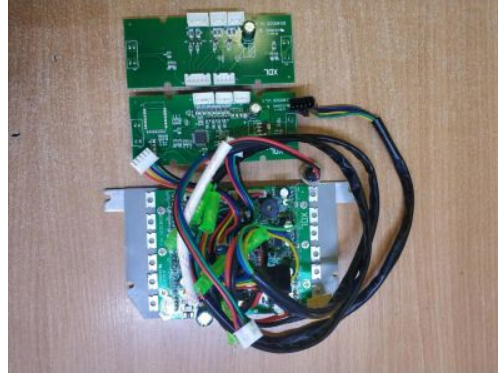
Figure 3.4: Factory hoverboard hub motor's controller
