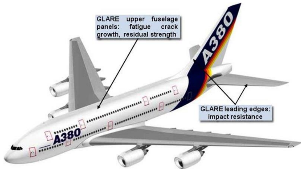
Figure 1.1. GLARE deployment in the Airbus A380 [1].
