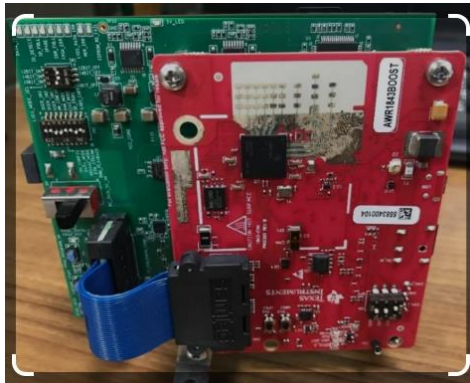
Fig 4.2. DCA 1000 EVM (Green) attached to the IWR 1843.
