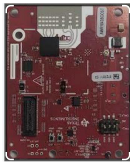
Fig 4.1. The millimeter wave radar sensor board.
