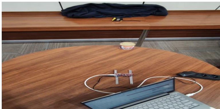
Fig 4.3. Millimeter wave radar setup to track object detection.
