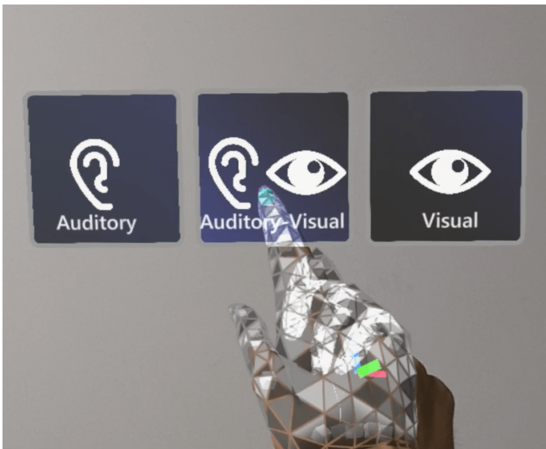
Figure 3.5: Holographic buttons for selecting the warning types with the MRTK holographic mesh overlaid to the hand
