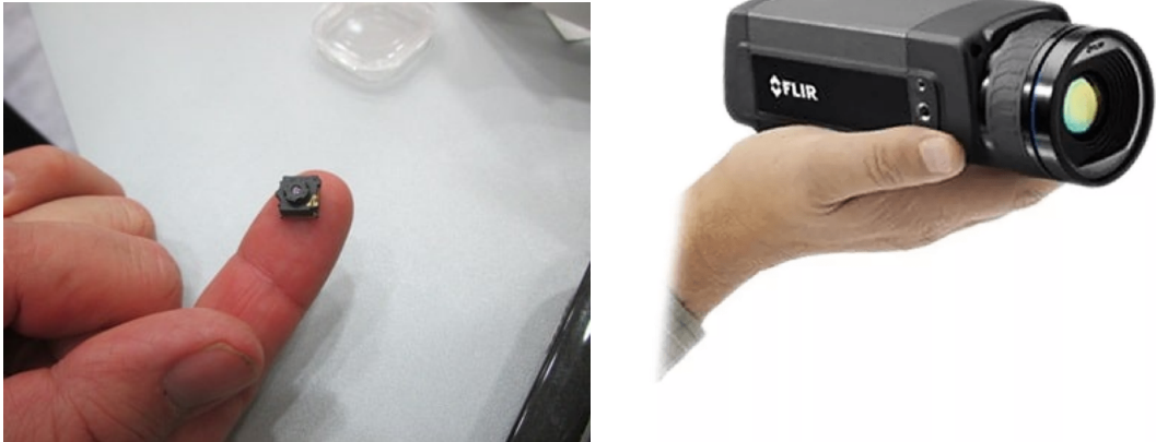
Figure 7.2: Thermal cameras compared to human finger and hand: a) Flir Lepton and b) Flir SC655
