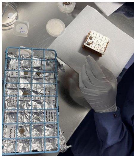
Figure 3-11. Sample installation for the XPS surveys
