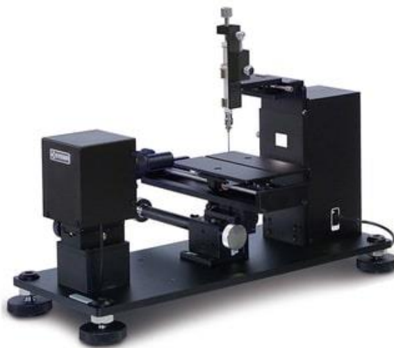
Figure 3-12. Contact angle measurement apparatus (OCA 15EC LMS instruments) used in this research work
