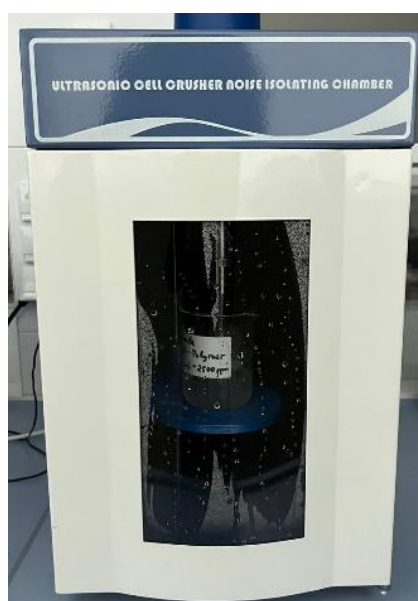
Figure 12. Ultrasonic cell crusher noise isolating chamber
